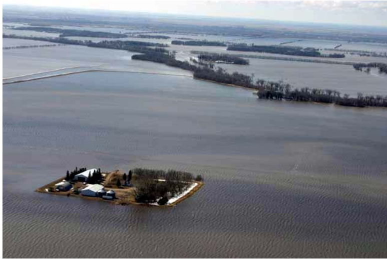
Farmstead ring dike located on the Tim Anvinson farm of Section 16, Higdem Township, Polk County, Minnesota. (Middle-Snake-Tamarac Rivers WD)
