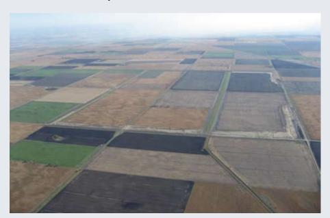
Aerial photo of the North Ottawa Impoundment project site looking south. The angle ditch near the bottom of the photo is the main outlet channel, JD No. 2.
